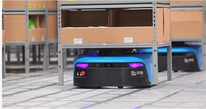
Automated (“Kiva”) Robot Systems
